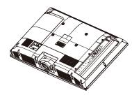
2 Secure the stand to the stand column on the TV with the six screws M4 type (16 mm) provided.
